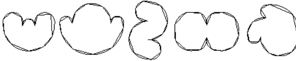
Figure 4.46: The difference between the original outlines and their polygonal approximations, i.e. an overlay of Figure 4.44 and Figure 4.45
